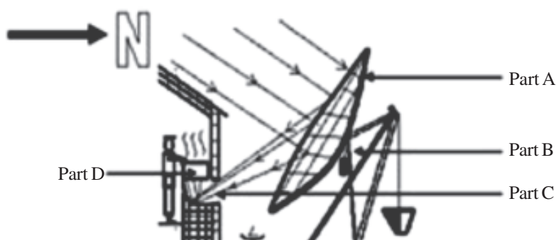
Fig. 31.6: Scheffler community cooker concentrator
